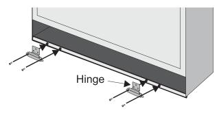
5) Place Bottom Frame near hinge. Flip hinge over Bottom Frame and secure with 3 screws.
